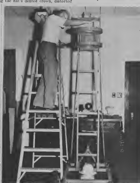
TO DETERMINE if a damaged safety hat can satisfactorily protect a man, the Equipment Inspection Group set up this test. The ball, dropped by J. E. Kirwin, struck each hat a 40-foot-pound blow.
